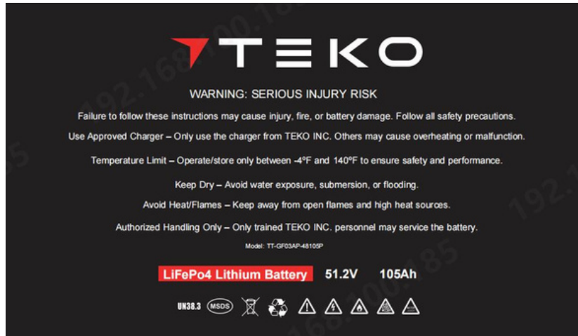
Battery Warning Decal
